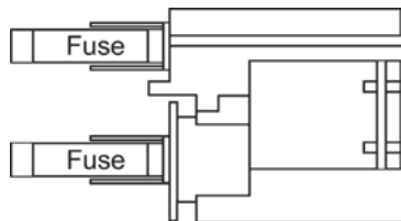
Fuse drawer for 220/240 voltage selection
